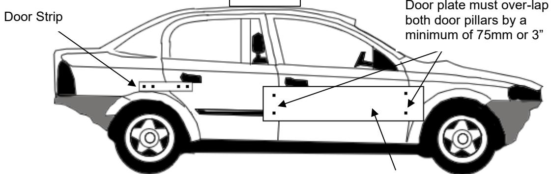
The Door plate must be fixed by either four 16mm or 19mm bolts or studs, through both the door pillars. No slotted holes allowed. **No welded plates are allowed to hold the door bar on.**
